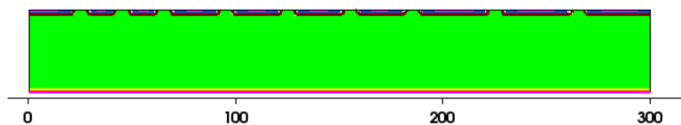
Figure 2. Circular geometry from Medici. 10 contacts in the radial direction to provide enough resolution for cluster area estimation. (Both radius and thickness is 300\ \mu\text{m} , no depletion region is showed.)
