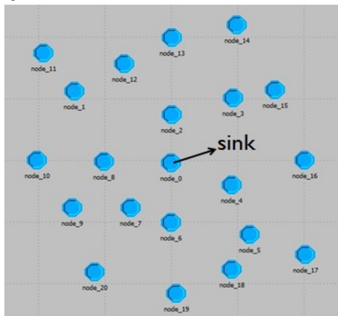
Figure 16: Square network topology used in the simulation
