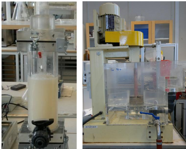
Fig. 1. Induced air flotation: a) customized 1 L cell (Zasadowski et al. 2012) and b) Voith cell
