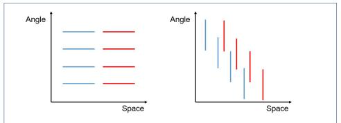
Figure 2: Phase space representation of light field camera sampling. Left: plenoptic 1.0; right: plenoptic 2.0.
