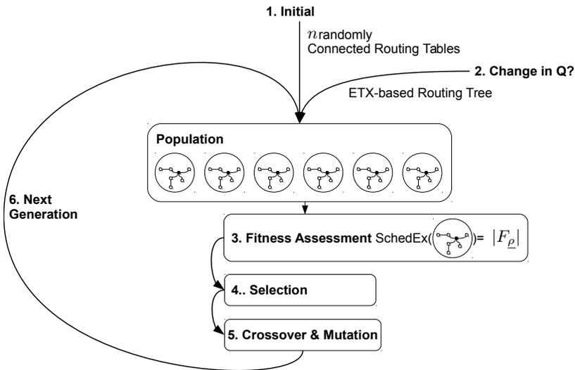
Figure 4.5: The GA algorithm loop for identifying valid and well performing network configurations that consist of a source-aware routing table and a slot-based schedule.
