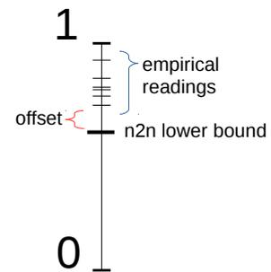
Figure 5.1: To provide valid end-to-end guarantees, the lower bounds for node-to-node PDRs that are used as a basis for scheduling and routing must consider an offset due to the stochastic nature of the channel.
