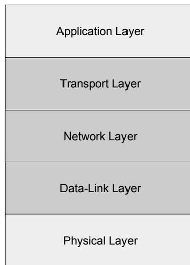
Figure 1.1: The generic WSN protocol stack. The means proposed in this thesis correspond to the dark grey layers.
