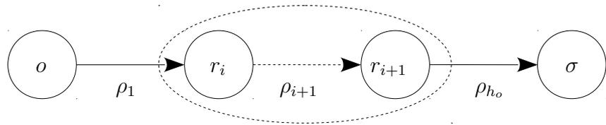
Figure 4.10: An exemplified routing path for all packets from origin  $o$  to sink  $\sigma$ , passing by  $i$  relays. The transmission on each link  $i$  must ensure the reliability  $\rho_i$  to fulfill the sensor-specific end-to-end demand of  $\underline{\rho}_o$ , according to (4.23).
