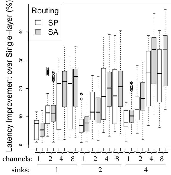
Figure 4.7: The improvement of the cross-layer GA over SchedEx based on heuristic routing. Source-aware routing can successfully be utilized, resulting in on average 9% better results if applied by the GA compared with single-path routing.
