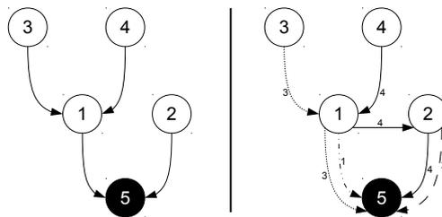
Figure 4.6: Single-path routing (left) vs. source-aware routing (right). For source-aware routing, transmissions are dedicated to a certain receiver, according to the source of the packet.
