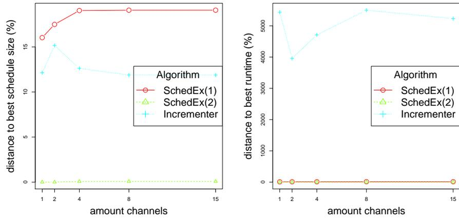
Figure 4.2: The average impact of the number of available channels on the scheduling performance (left) and runtime (right) for the three reliability-aware approaches. SchedEx(2) produces the shortest schedules throughout the investigation. The Incrementer is the algorithm presented in [YLH<sup>+</sup>14].
