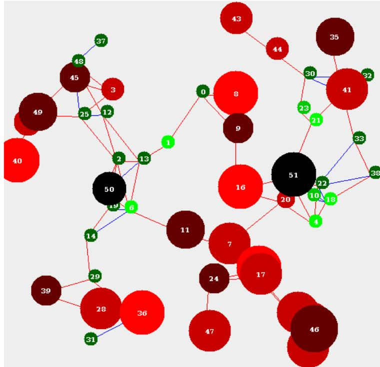
Figure 4.12: An example of visualizing sensors with deadline misses (red), those without (green), and sinks (black). The size of the sensors stands in relation to the number of missed packets, and the lightness of the colour illustrates its urgency. For the given case, a sink deployment in the lower-right corner could be investigated to resolve the deadline misses there.
