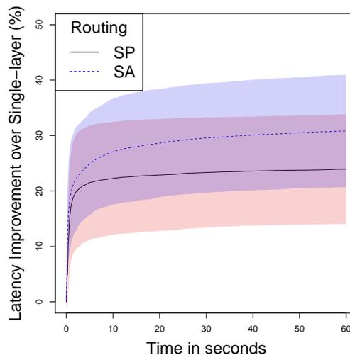
Figure 4.8: The average convergence improvement of the cross-layer GA over SchedEx using heuristic ETX-based routing.
