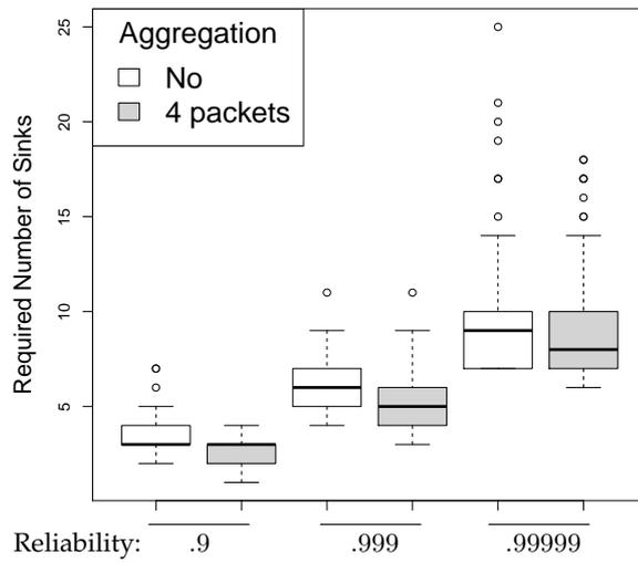
Figure 4.13: A box-plot visualizing the impact of aggregation, summarized over all channel models. Aggregation gives an improvement of in average ca. 10%.
