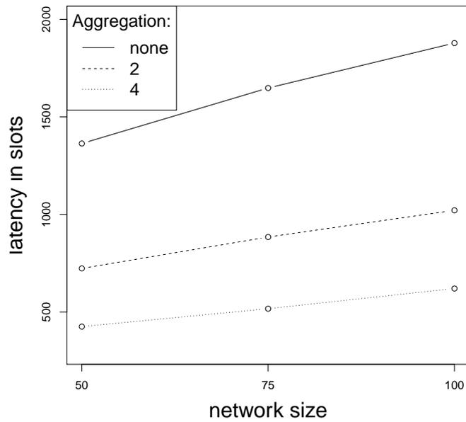
Figure 4.4: The aggregated average required frame size for the topologies to submit all packets to the sink given an end-to-end reliability constraint of 99.999% using SchedEx and a maximum aggregation of four packets. The improvements for an aggregation of 2 and 4 packets are significant.
