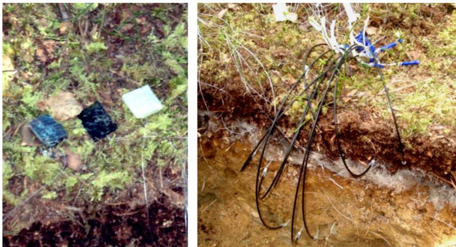
**Figure 12.** Photos of the three amended minerals apatite, biotite and oligoclase (left), and the soil installation of mineral samples and tension-lysimeters in the O, E and B horizons of a podzol soil (right).
