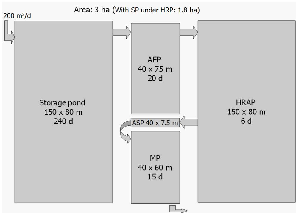
Figure 3. A pond system designed for 200 m<sup>3</sup>/d load of wastewater, and a storage time of 8 months, 240 days, meaning that the High Rate Algae Pond (HRAP) is only active for 4 months during the summer period. Other abbreviations, see Figure 1.
