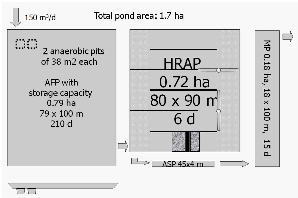
Figure 2. A pond system designed for 150 m<sup>3</sup>/d load of wastewater, and a storage time of 7 months, 210 days, meaning that the High Rate Algae Pond (HRAP) is only active for 5 months during the summer period. The HRAP has a paddlewheel with concrete reinforcement in the bottom down in the picture. To the right it also has swinging walls, enabling flexibility in the HRP volume. Other abbreviations, see Figure 1.
