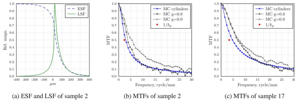
Fig. 1. Simulated ESF and corresponding LSF in (a) and simulated MTFs for single paper sheet sample 2 in (b) and sample 17 in (c). The main difference between the samples is that sample 17 has a about four times larger scattering coefficient compared to sample 2. The red dots indicate the measured value of  $k_p$  presented by Arney et al.
