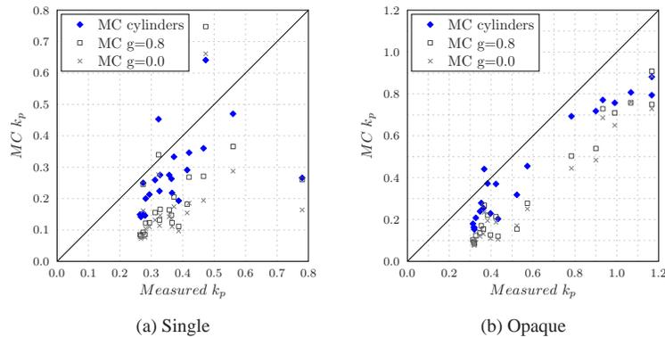
Fig. 2. Measured values of  $k_p$  versus simulated values for a single sheet (a) and an opaque pad of sheets (b).
