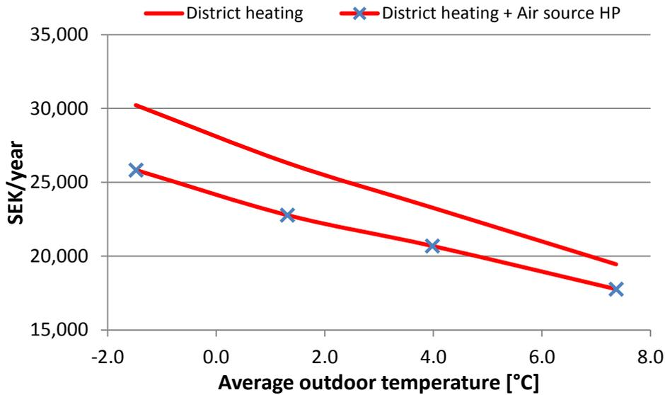
Fig. 7. The yearly costs including material, installation, maintenance, and energy costs for heat supplied from the district heat and heat supplied from both the district heating and air-source heat pump.
