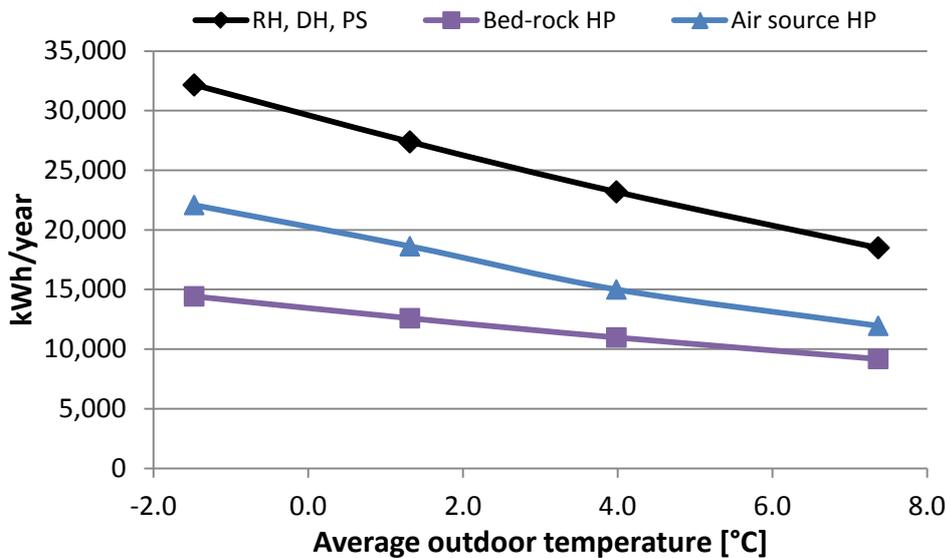
Fig. 8. Final energy use by different heat technology sources and in different climate conditions
