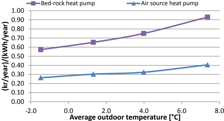
Fig. 6. A comparison of the cost of each unit of final energy saved between air-source and bed-rock heat pumps in different climate conditions.
