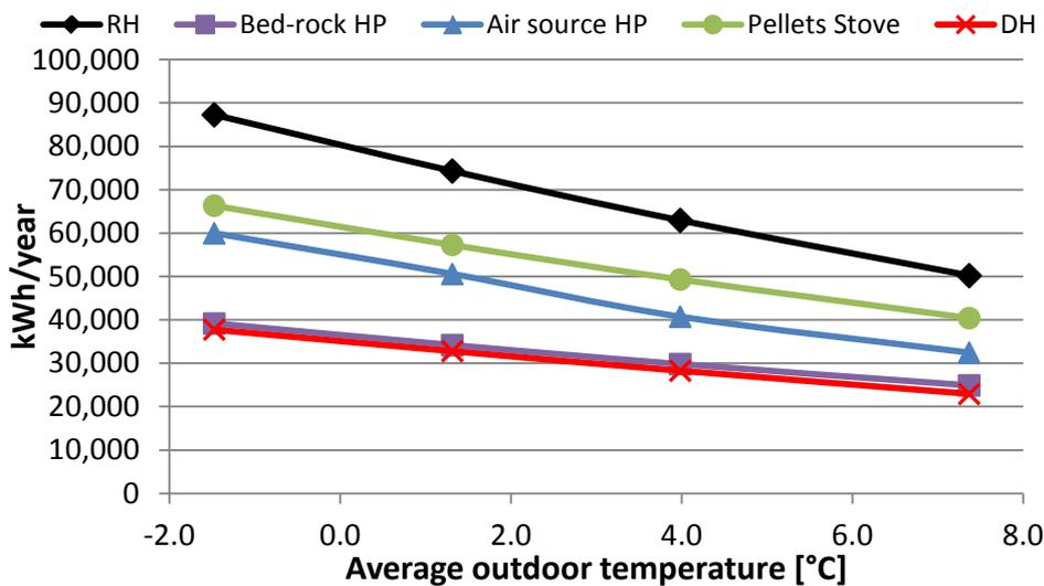
Fig. 4. The primary energy use for different heat source technologies and in different climate conditions
