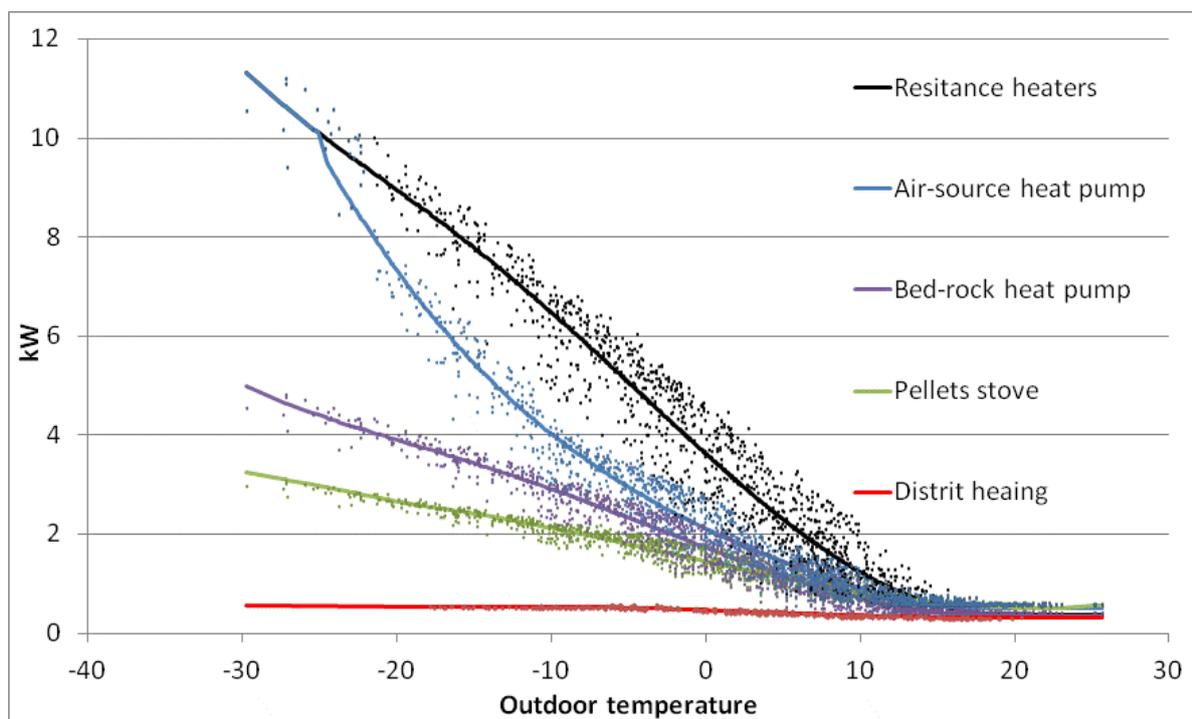
**Fig. 2. The electricity production load that is needed to provide similar indoor conditions by different heat source technologies and for different outdoor temperatures in the case study building.**
