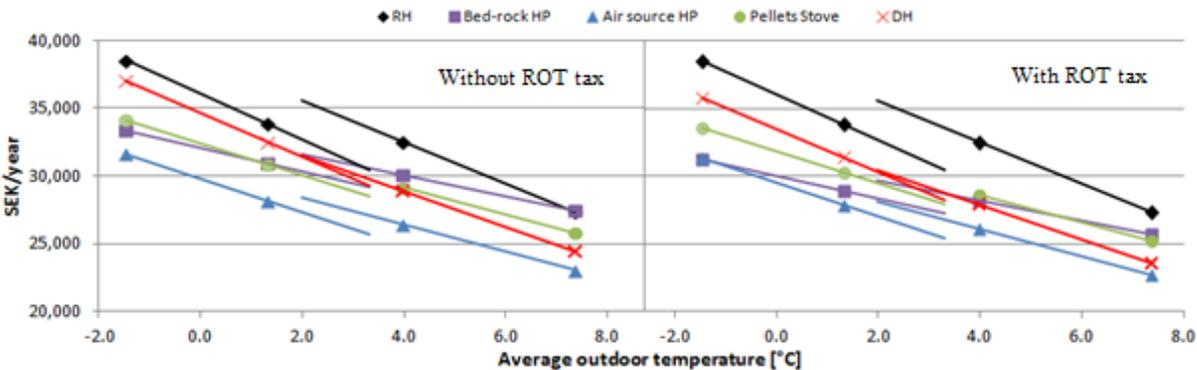
Fig. 5. The yearly costs including material, installation, maintenance, and energy costs for different heat source technologies and climate conditions with and without the Swedish ROT tax.
