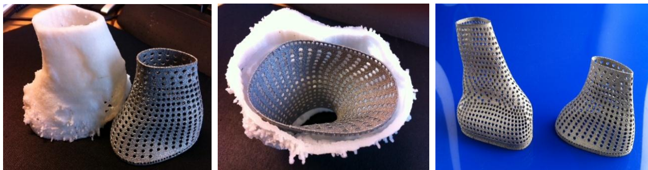
Fig. 7 Metal cages made from medical grade Ti6Al4V using EBM ® technology are designed to reinforce the patient's femur, ready to accommodate traditional knee replacement implant
