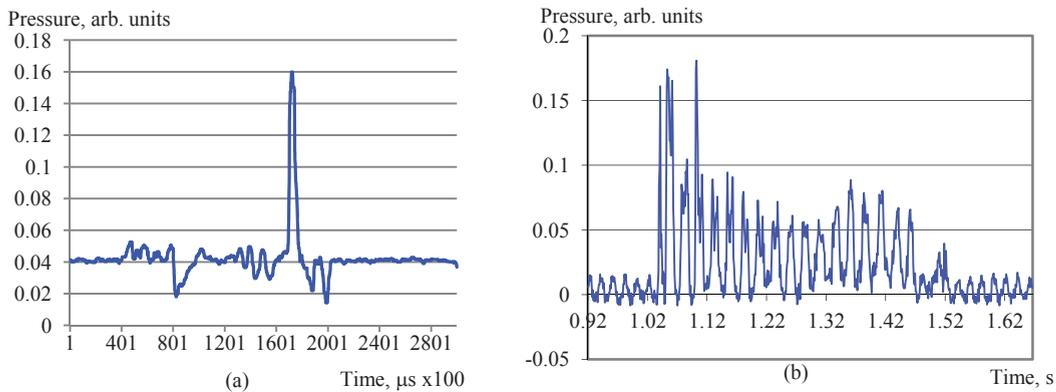
Fig. 2. (a) Time dependence of the pressure inside the snow under the ski track; descend #6, ski pair 112 [4], both front and rear signals are visible. (b) Pressure signals from the pressure sensor on the snow, when static skier is 'stamping' over the sensor
