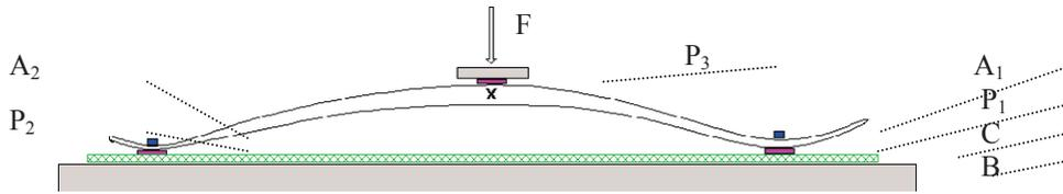
Fig. 3. Setup for the studies of the forced vibrations of the loaded cross-country skis. P<sub>1</sub>, P<sub>2</sub>, P<sub>3</sub>- thin film pressure sensors; A<sub>1</sub>, A<sub>2</sub> – accelerometers; F- static load and harmonic excitation; C- acoustic insulation, B- solid base
