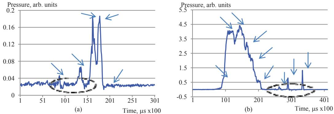
Fig. 1. Time dependence of the pressure between the skis and the snow; field experiments, descend #39, pair 105 [4] from the front of the right ski (a) and the rear of the same ski (b). Corresponding oscillations are marked by arrows and the incidents, when parts of the skis are losing contact with the snow are marked by dashed lines. Signal (b) is coming 100 ms after signal (a)
