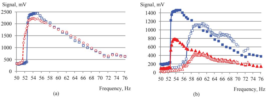
Fig. 4. Frequency dependence of the peak-to-peak magnitudes of the acceleration signal components normal to the ski surface. (a) Front of the ski, frequency is swept up (squares, solid line) and down (circles, dotted line); (b) Front of the ski (squares) and back of the ski (triangles), with different excitation amplitude. Solid squares and circles correspond to 60% higher excitation signal amplitude
