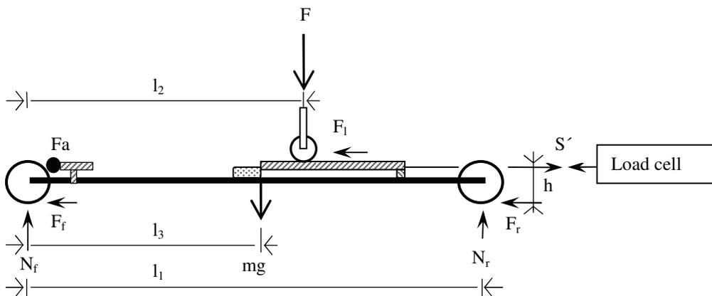
Fig. 1 Free body diagram of the experimental setup.
