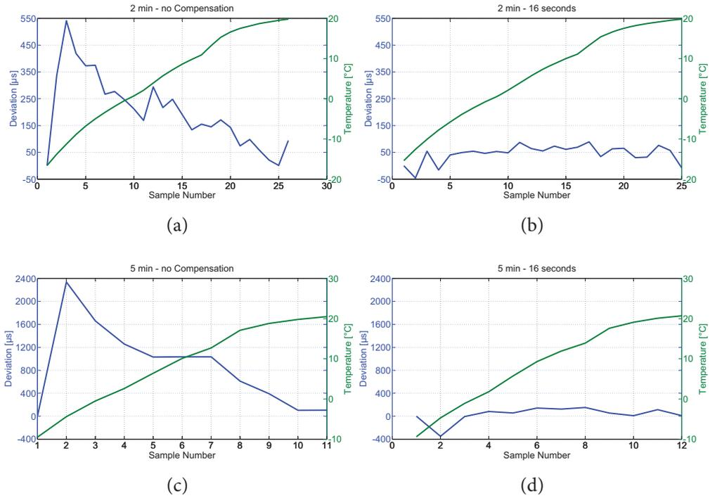
Figure 2.12: Measurement of wake-up accuracy under changing temperature conditions after cooling in the freezer – (a) 2 min synch. interval, uncompensated; (b) 2 min synch. interval, compensated; (c) 5 min synch. interval, uncompensated; (d) 5 min synch. interval, compensated
