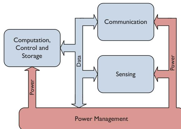
Figure 2.1: Abstract architecture of typical sensor nodes, used in Wireless Sensor Networks
