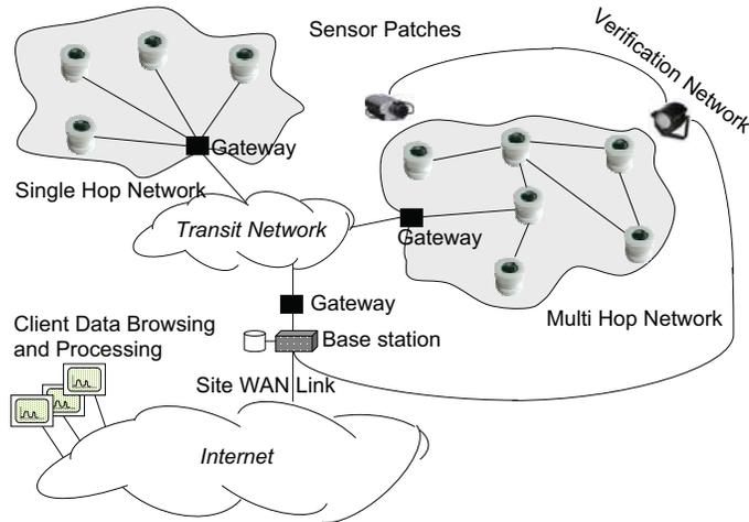
Figure 1.3: System architecture of the Wireless Sensor Network deployed on Great-Duck-Island in 2003 [15]
