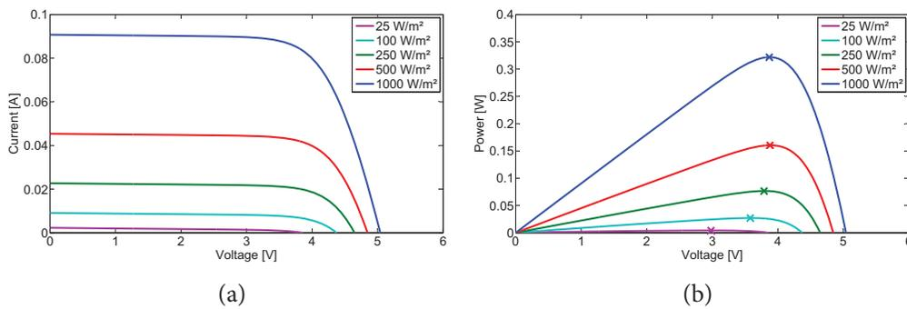
Figure 3.5: Solar panel characteristics of a 450 mW panel with 9 cells in series at different irradiance levels – (a) I-V characteristic and (b) P-V characteristic
