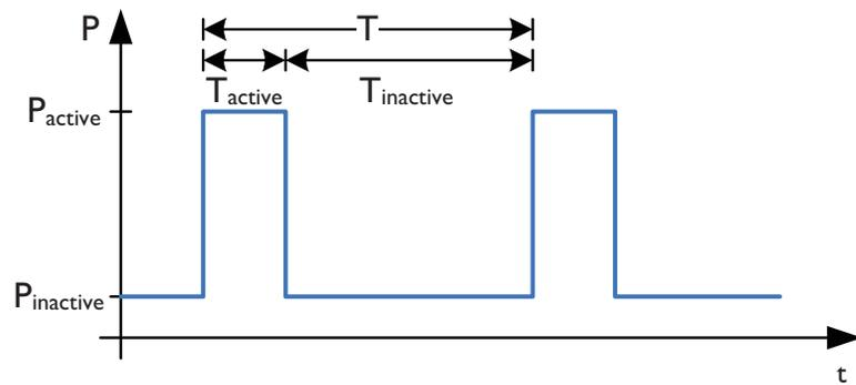
Figure 2.2: Graphical representation of the duty-cycling principle (simplified for bi-modal operation states)
