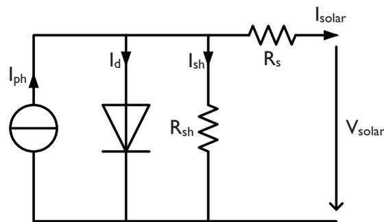
Figure 3.13: Equivalent circuit of a solar panel according to the single-diode model
