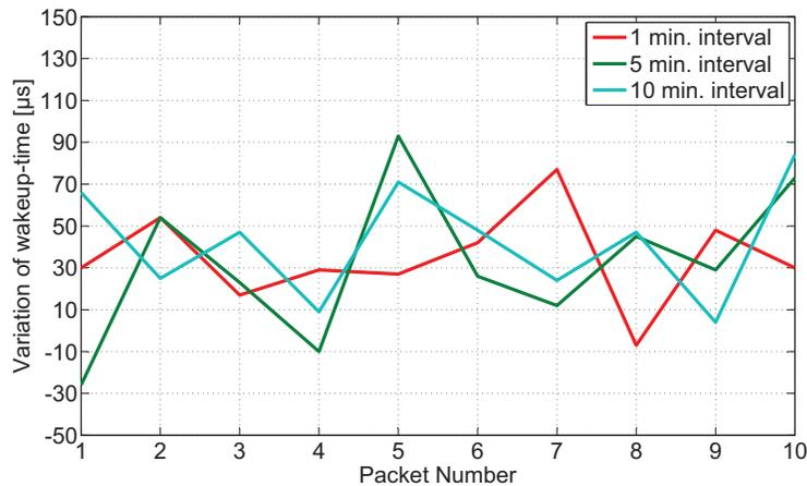
Figure 2.10: Deviation of measured to scheduled time interval between *radio-ready-to-receive* and synchronization message reception for different synchronization interval length
