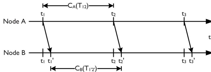
Figure 2.8: Timeline of an interval-measurement based synchronization method
