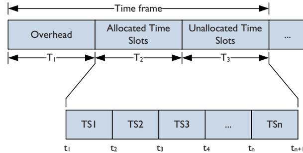
Figure 2.5: Typical structure of a TDMA based communication schedule
