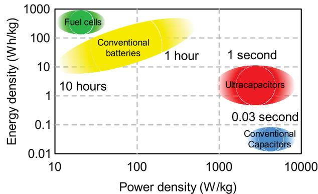
Figure 3.4: Classification of energy density and power density of energy storage devices [49]
