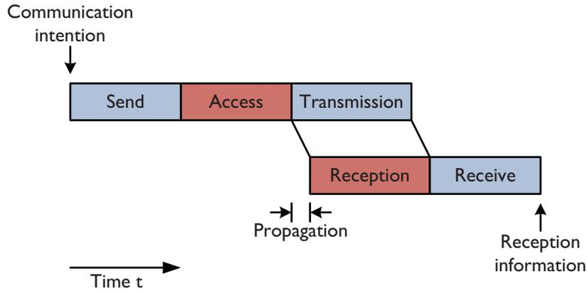
Figure 2.6: Occurrence of delay components during a packet transmission between two nodes in a Wireless Sensor Network
