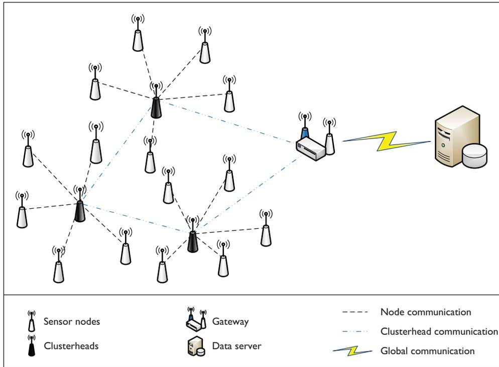
Figure 1.2: Typical network architecture of environmental monitoring applications under scope
