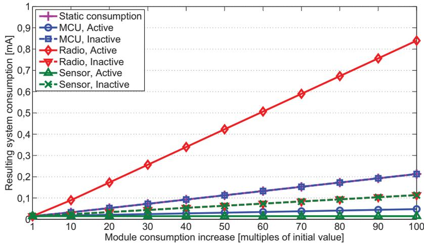
Figure 2.3: Influence of the consumption per module on the overall duty-cycled system consumption. Consumption increase can mean both, increase in amplitude and increase in time period
