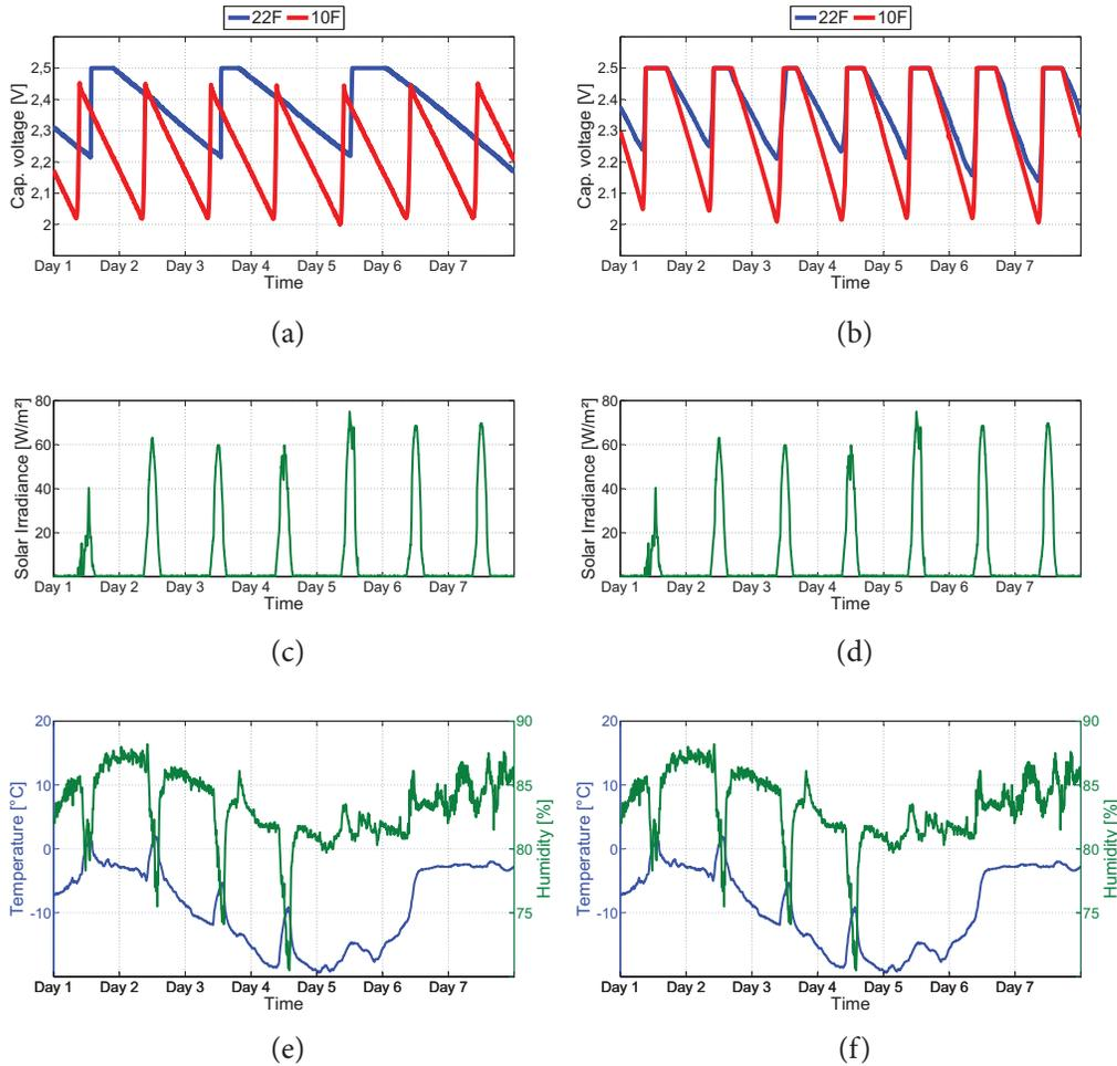
Figure 3.10: System behavior of two solar energy harvesting architectures during one week of deployment – (a),(b) capacitor voltage levels for directly-coupled architecture (left column) and LDO-based architecture (right column); (c),(d) irradiance conditions during the week; (e),(f) temperature and humidity during the week
