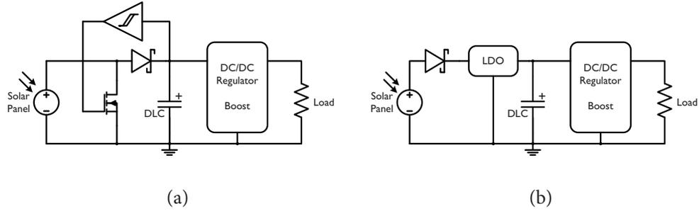
Figure 3.8: DLC-based solar energy harvesting architecture implementations – (a) directly coupled architecture and (b) architecture with LDO input regulation
