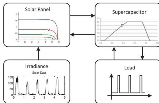
Figure 3.12: Overview of energy-related interactions between modules of the solar energy harvesting system, based on a directly-coupled architecture
