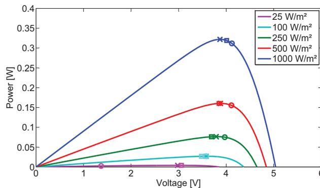
Figure 3.6: Accuracy of MPPT based on fractional open-circuit voltage and fractional short-circuit current; real MPP marked by cross, estimated from  $V_{oc}$  marked by squares, estimated from  $I_{sc}$  marked by circles
