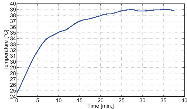
Figure 2.13: Measurement of in-box temperature of a light-colored plastic enclosure under direct sunlight in summer conditions; location Sundsvall/Sweden; measurement with on-board temperature sensor [42] of Sentio-e<sup>2</sup>, 1 Hz
