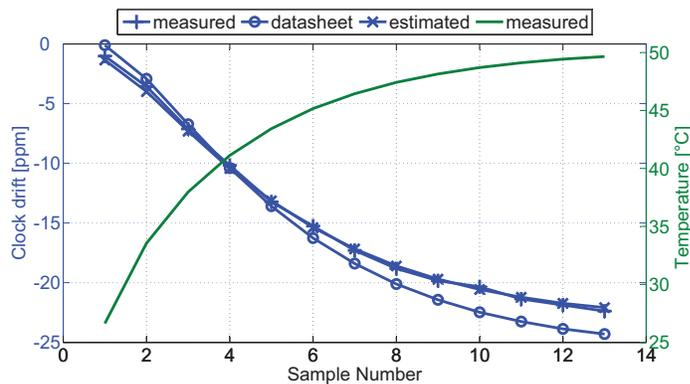
Figure 2.14: Comparison of measured, estimated and datasheet temperature drift behavior; measured with on-board temperature sensor of Sentio-e<sup>2</sup>; determined from drift over 1 minute while heated in an oven
