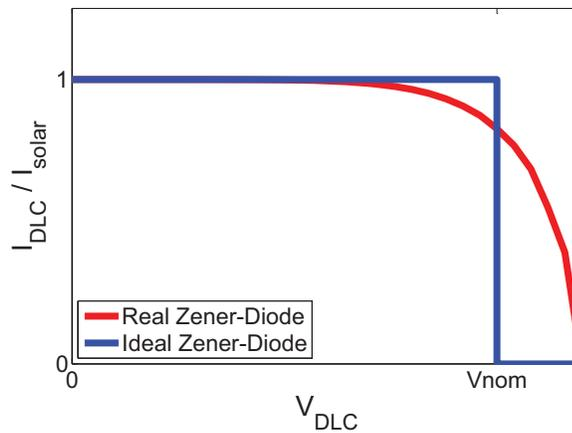
Figure 3.9: Behavioral comparison of ideal and real zener-diode characteristics
