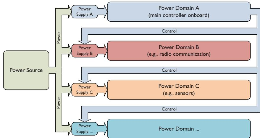
Figure 2.4: Principle of different power domains for dynamic adjustment of power consumption and on-demand performance
