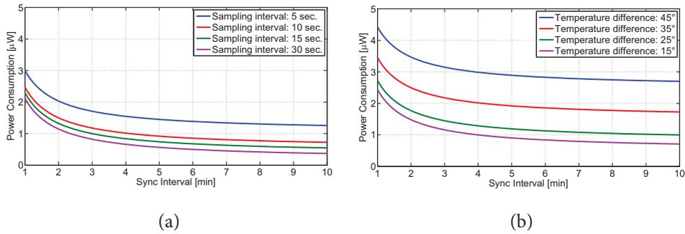
Figure 2.15: Comparison of power consumption needed to deal with temperature drift – (a) Temperature compensation with different temperature sampling rates; (b) Extending reception guard-time for different maximum deviations from the turnover temperature
