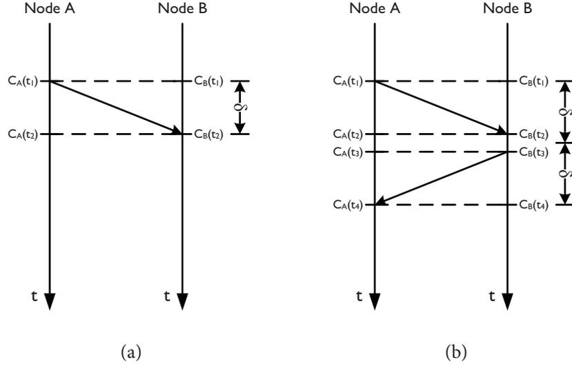
Figure 2.7: Underlying timeline of packet transmission for (a) unilateral synchronization method and (b) bidirectional synchronization method
