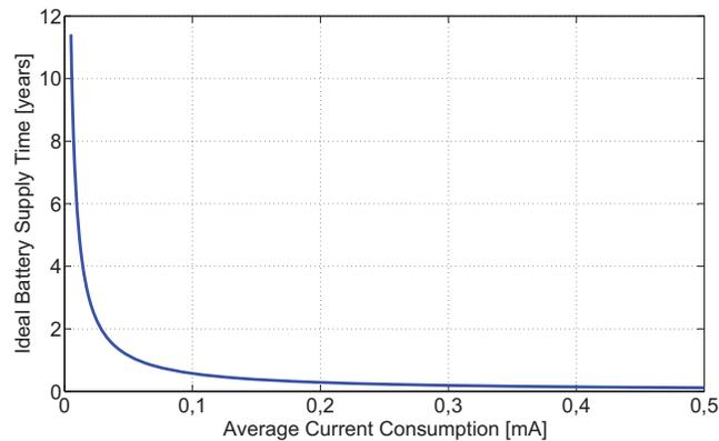
Figure 3.1: Simplified energy supply time from an AA-type battery in ideal situation
