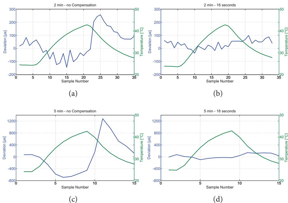
Figure 2.11: Measurement of wake-up accuracy under changing temperature conditions in the oven – (a) 2 min synch. interval, uncompensated; (b) 2 min synch. interval, compensated; (c) 5 min synch. interval, uncompensated; (d) 5 min synch. interval, compensated
