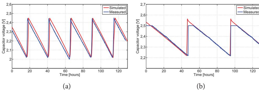
Figure 3.16: Evaluation of energy levels estimated by the system model compared to deployment results – configured with (a) a 10 F DLC and (b) a 22 F DLC
