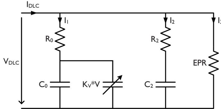
Figure 3.14: Equivalent circuit of a Supercapacitor according to the two-branch model
