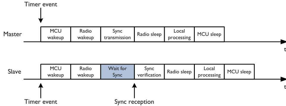
Figure 2.9: General sequence of tasks performed by synchronization master and slave at the beginning of each communication frame
