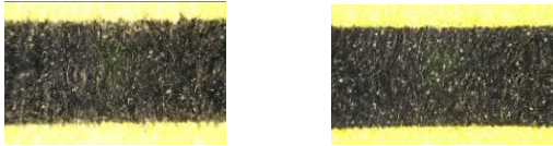
Figure 6. A horizontal printed line on a yellow background printed on the paper sample without surface fixation, sample G (left image) and paper with a high level of surface fixation, paper J (right image)
