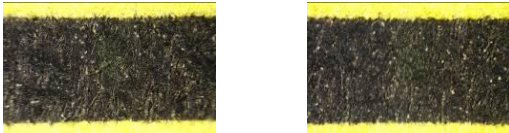
Figure 5. A horizontal printed line on a yellow background printed on paper B (left image) and paper A(right image)
