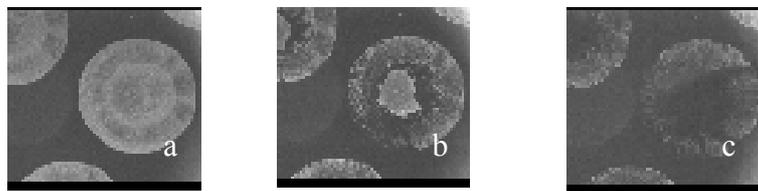
**Figure 2.** Three images collected during ink detachment of flexographic ink on cellulose surface. a) 1 second, b) 11 seconds and c) 13 seconds exposure of basic water solution (pH 11.5). These measurements were collected from experiments with an initially dry cell.
