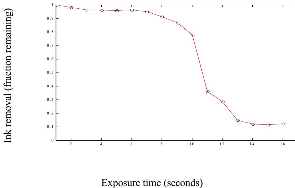
**Figure 4.** Flexographic ink removal from cellulose surfaces as determined from binary images.
