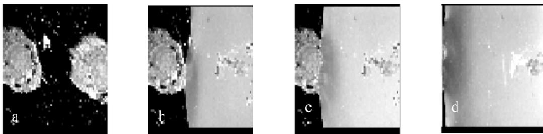
**Figure 3.** Offset ink detachment from cellulose surface. Images were collected during the experiment. a) Dry cellulose surface with two printed offset dots. b-d) Water (with a brighter shade) is gradually covering the cellulose surface. The print is released when the water reaches the dry print. These measurements were collected from experiments with an initially dry cell.
