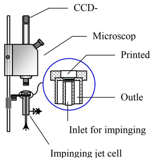
**Figure 1.** Schematic description of the Impinging jet equipment
