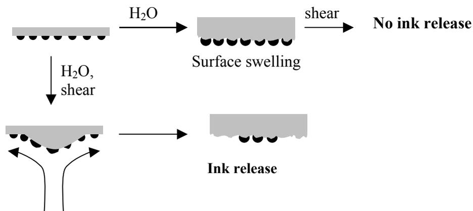
**Figure 6.** Schematic representation of ink removal of offset print from a cellulose surface. No ink was removed when the surface was pre-wetted but a combination of surface swelling and shearing was sufficient to remove the ink.
