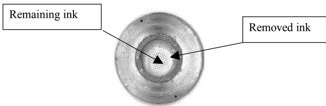
**Figure 5.** Offset ink removal from the model cellulose surface.
