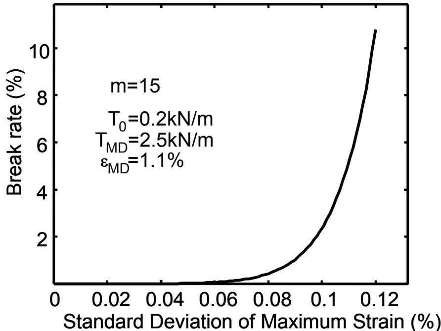
**Figure 10** Break rate as a function of standard deviation of maximum strain deviation
