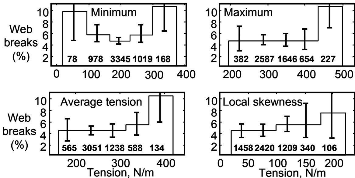
**Figure 17** Effects of web tension nonuniformity on web breaks in pressroom.
