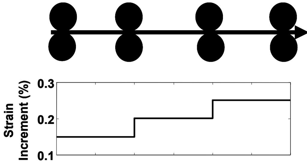
**Figure 7** Web strain changes at printing nips.
