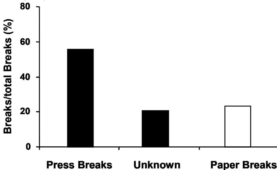
Figure. 4 Break cause statistics (Coldset press printing newsprint)
