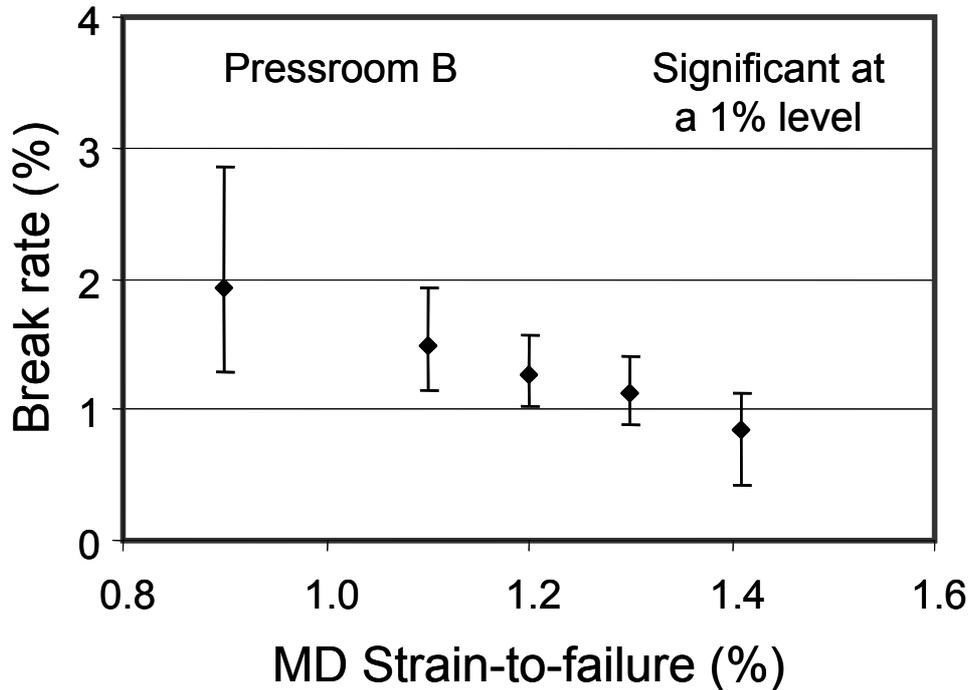
Figure 13 Break rate plotted against the machine direction strain-to-failure.
