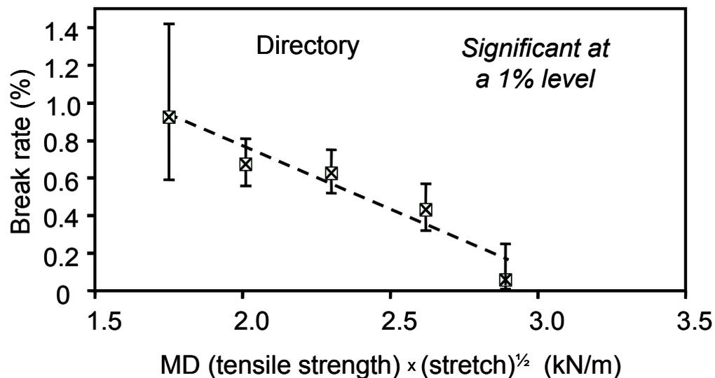
**Figure 16** Break rate plotted against a combined parameter. TEA is often mentioned as a predictive parameter of web breaks since it is phenomenologically related to both tensile strength and strain to failure. The analyses of mill and pressroom data [5, 7] indeed showed that TEA has a good association with web breaks in pressrooms, although the consistency is not as high as the one for tensile strength.
