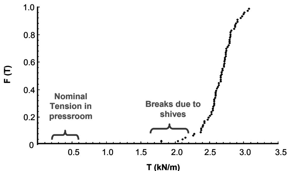
**Figure. 6** Strength Distribution of Newsprint.  $F(T)$ : Cumulative probability density function (the probability that paper breaks less than tension  $T$ ),  $T$ : Tension per unit width
