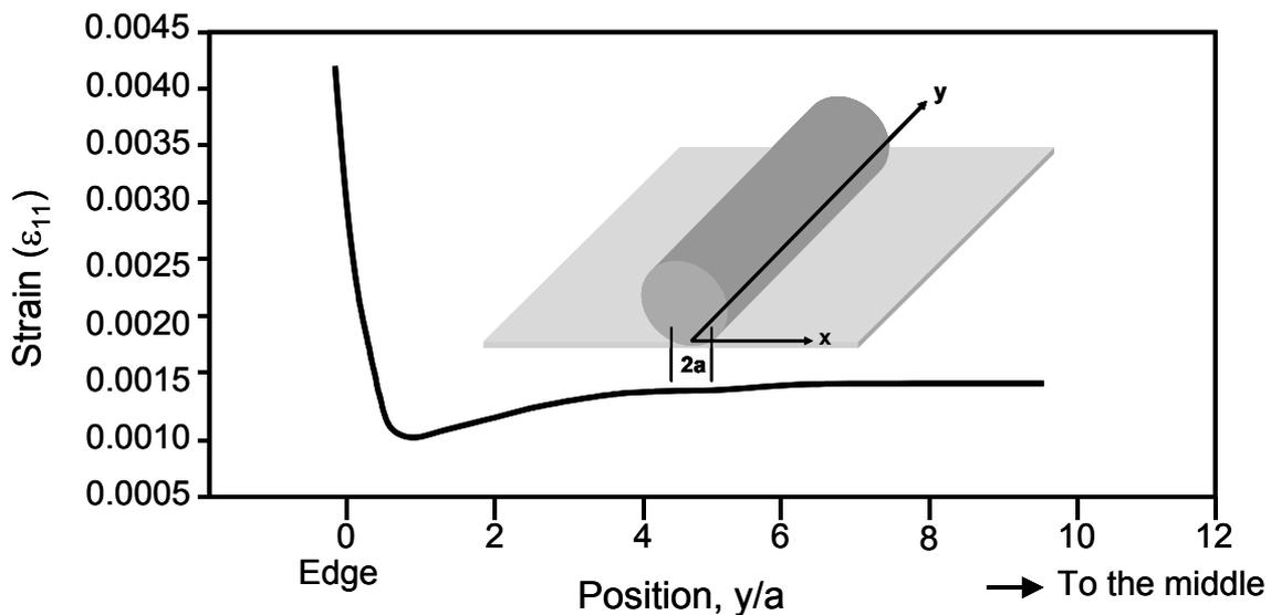
**Figure 8** The distribution of the machine direction normal strain of paper along the roll axis direction. The strain is taken at the middle of the nip.  $y$ : Distance from the roll edge,  $a$ : A half nip width
