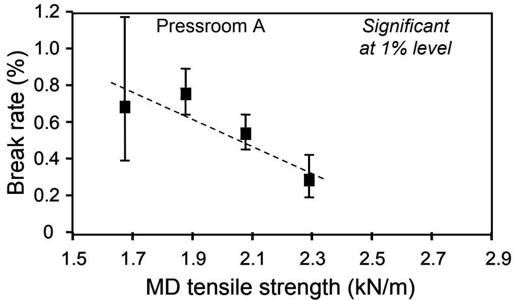
Figure 12 Break rate plotted against the machine direction tensile strength.
