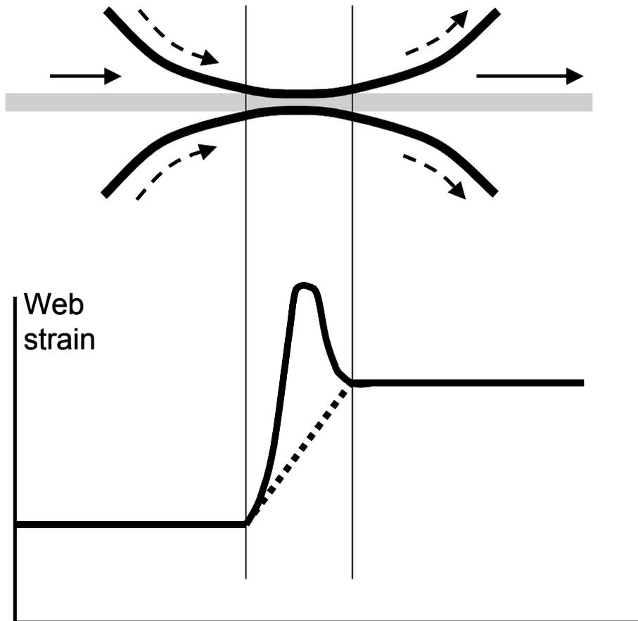
**Figure 9** Change in web strain in the printing nip. When there is a difference in web speed before and after the nip, the web undergoes a strain change (dotted line). In addition the nip impression causes expansional strain in the paper. The total effect is represented by the solid line.
