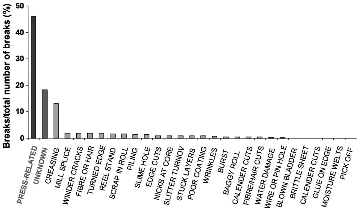
Figure. 3 Break cause statistics (Heatset offset press)
