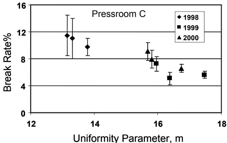
**Figure 14** Break rate plotted against the strength uniformity parameter, m
