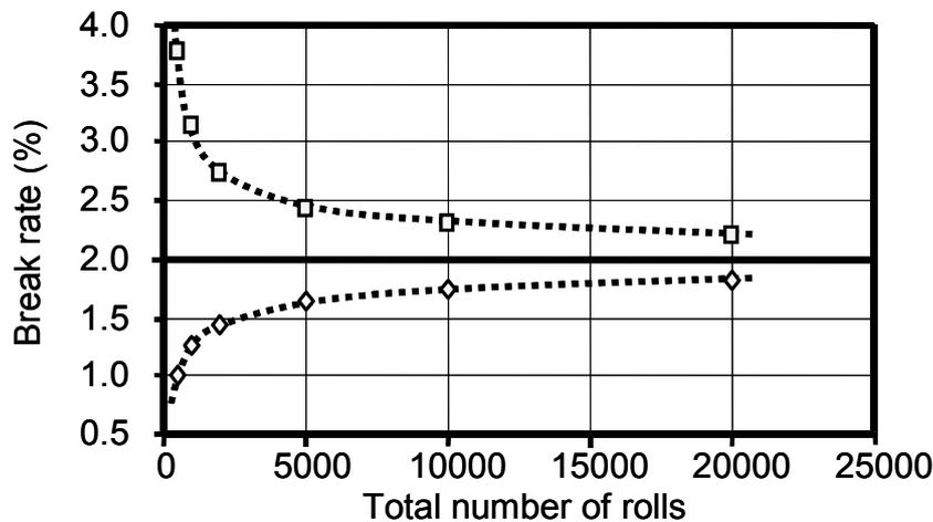
**Figure 1.** Upper and lower bounds of 95% confidence interval as a function of the number of rolls observed for the average break rate 2%.
