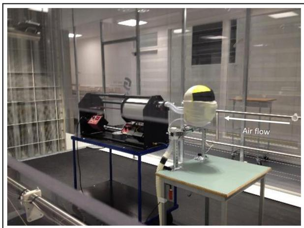
**Figure 2.** Experimental setup of measurements of resistance to breathing: the mechanical lung simulator, a head made from ABS plastic with mounted foam sheet on the face and one type of heat and moisture exchanger tested in the study.
