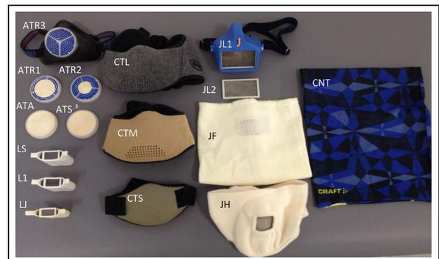
**Figure 1.** The heat and moisture exchangers with different filters tested for resistance to breathing: Airtrim with five different filters – ATA, ATS, ATR1, ATR2, ATR3; Lungplus in three different variants – LS, LI, LJ; CT Mask in three different sizes – CTL, CTM, CTS; Jonaset with two different filters – JL1, JL2, and two face tubes with filters – JF, JH; Craft, a neck/face tube without any filter – CNT (Table 1).
