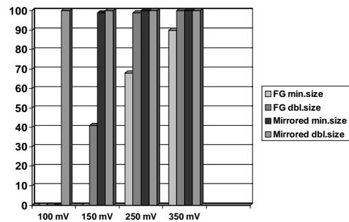
Fig. 6. Bargraph showing Yield for FGMOS and Mirrored gate with minimum and double minimum sized transistors for different power supplies.
