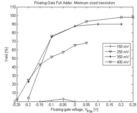
Fig. 4. Yield for a floating-gate full-adder working in subthreshold with different  $V_{dd}$  and  $V_{FGp}$ . Minimum Transistor sizes have been used.
