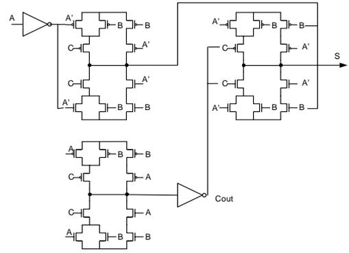
Fig. 3. Mirrored gate Full Adder topology.
