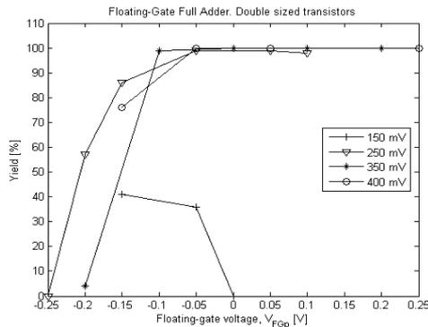
Fig. 5. Yield for a floating-gate full-adder working in subthreshold with different  $V_{dd}$  and  $V_{FGp}$ . The transistor lengths and widths have been double minimum size design.
