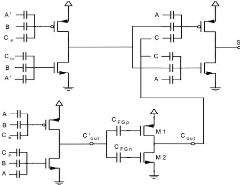
Fig. 2 Full-Adder design with the floating-gate elements.
