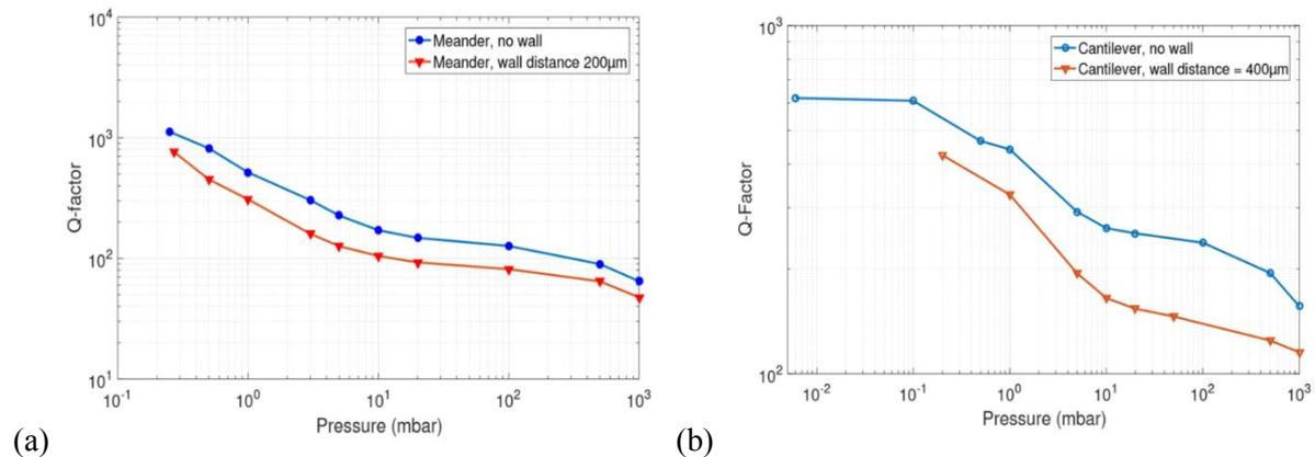
Figure 6. Q-factor for (a) meander and (b) cantilever as a function of pressure with and without wall.
