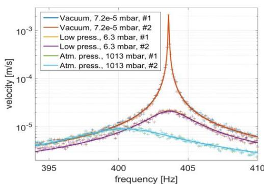
Figure 5. Measurement data (crosses) and fitted curves (solid lines) for the meander structure at three different pressures
