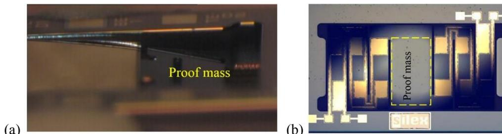
Figure 3. Image of MEMS (a) cantilever and (b) meander structure with proof mass.
