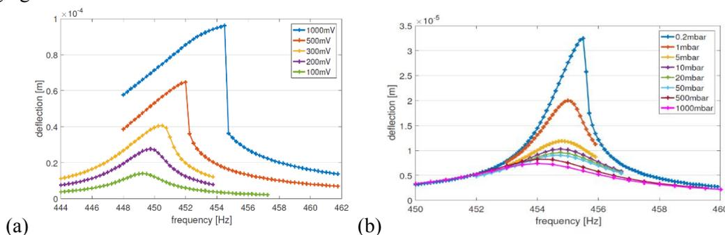
Figure 4. Spectra for the first resonance peak measured with the single frequency sine sweep method of MEMS cantilever as function of frequency and (a) excitation amplitudes in air, (b) pressure in the vacuum chamber with the excitation amplitude of 100mV.
