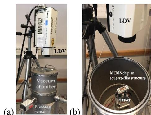
Figure 1. (a) Image of the experimental setup to estimate the energy losses showing the LDV with a special objective that allows measurements of MEMS structures. Below the LDV, the vacuum chamber is seen. The measurement is made through the glass window. (b) View of the small-size shaker inside the vacuum chamber with a MEMS chip on the sample holder.
