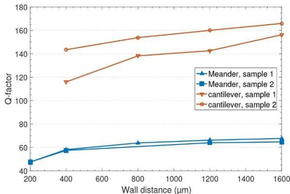
Figure 7. Q-factor as a function of the wall distance for cantilever and meander samples at 1000 mbar.
