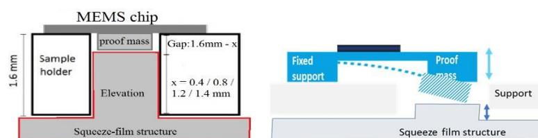
Figure 2. Sketch of the elevation module placed under sample for squeeze film damping experiments.
