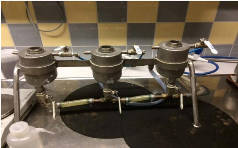
Fig 5- The equipment used for the determination of the Water retention value (WRV) at the SCA R&D Centre.
