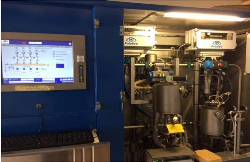
Fig 8- The PulpEye instrument used to determine fibre characteristics at the SCA R&D Centre.
