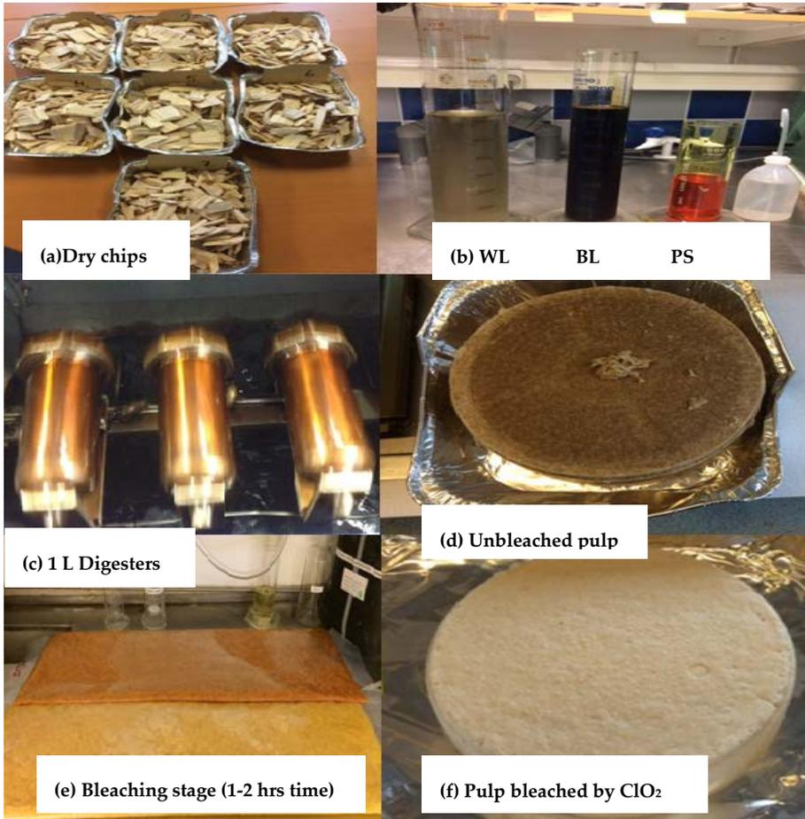
Fig 4- Some images of kraft pulp (from chips to bleached condition) taken, at the SCA R&D centre.
