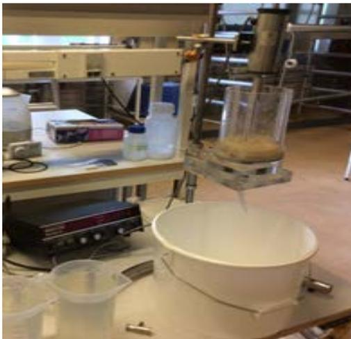
Fig 9- Specially- designed Britt Dynamic Drainage Jar (BDDJ) used at the SCA R&D Centre.
