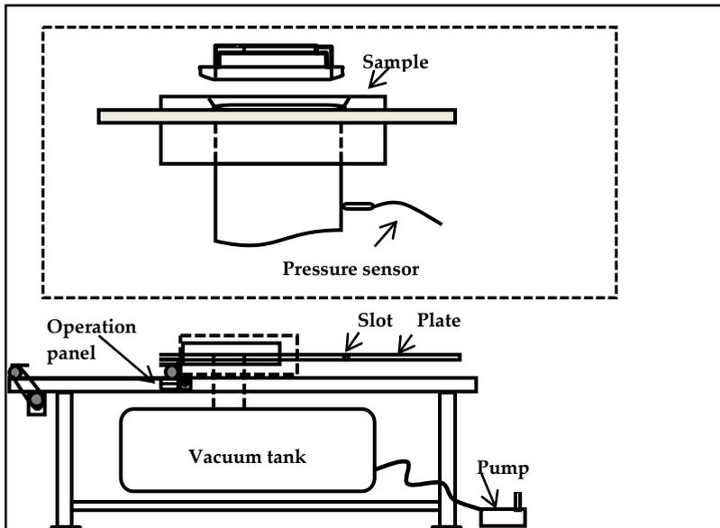
Fig 10- The vacuum dewatering apparatus (redrawn from Granevald et al. 2003).
