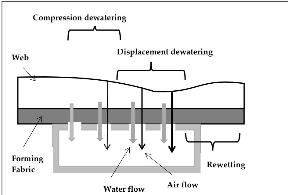
Fig 3- The mechanism of suction box dewatering (Redrawn from Åslund and Vomhoff 2008)
