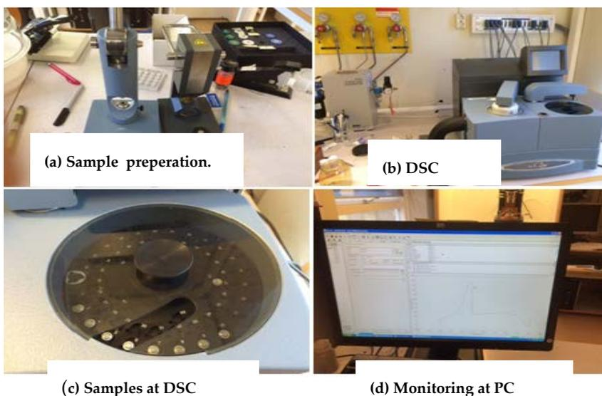
Fig 7- Analysis of pore volume by DSC at different stages (images a- d) at RISE Bioeconomy.
