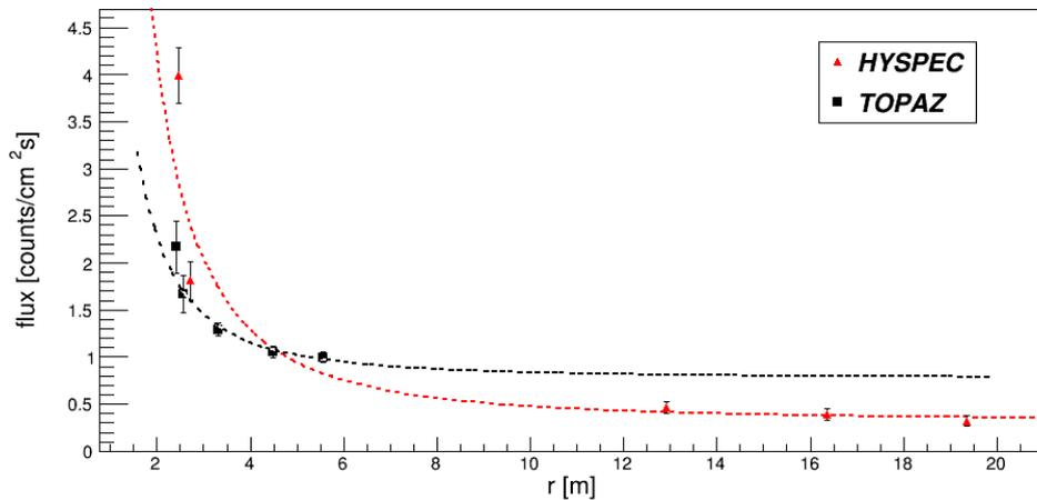
Figure 3: Neutron fluxes measured with the Arktis NDT as a function of distance from the monolith biological shielding for the HYSPEC and TOPAZ beamlines.
